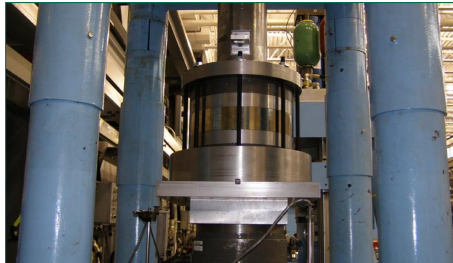
Figure 2. A picture of the full damper on its 100 kip (4.5 kN) actuator test rigging
